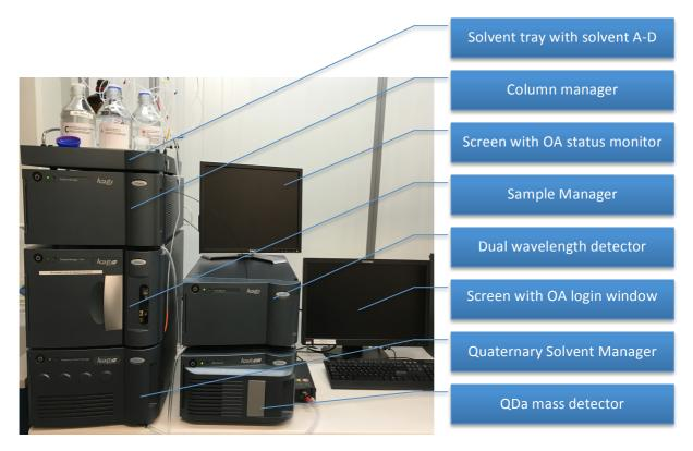
The two-stack system shown above consists of a left stack comprising (from top to bottom) solvent tray with solvents A-D, a Column Manager (= column oven) with two different columns, a Sample Manager – FTN (= autosampler), and a Quaternary Solvent Manager (= pump) and a right stack comprising a TUV Dual Wavelength detector and a QDa single quadrupole mass detector.
