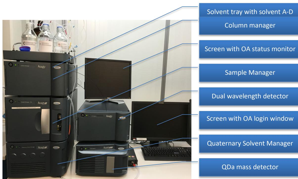
The two-stack system shown above consists of a left stack comprising (from top to bottom) solvent tray with solvents A-D, a Column Manager (= column oven) with two different columns, a Sample Manager – FTN (= autosampler), and a Quaternary Solvent Manager (= pump) and a right stack comprising a TUV Dual Wavelength detector and a QDa single quadrupole mass detector.
